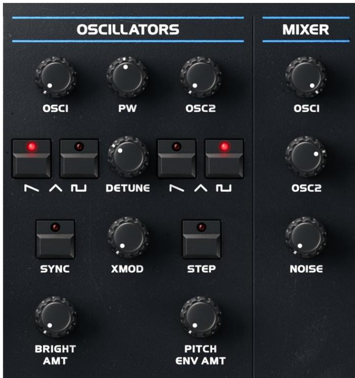
In the OB-X cross modulation (Frequency Modulation), OSC2 modulated OSC1. On the OB-Xd this is reversed: OSC1 modulates OSC2. Sounds created by sync and x-mod this way were judged more useful than the in-harmonic results of the original modulation path.
