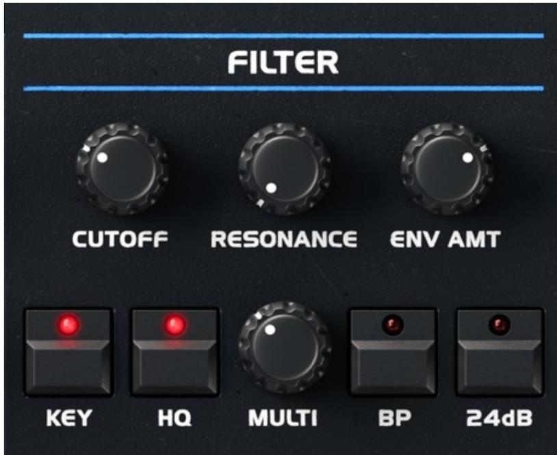
It implements a Multi-mode 12dB/octave filter like the Oberheim SEM module. Using the **MULTI** rotary control, you can crossfade between low-pass behavior on the complete left, to either notch (by default) or bandpass (using the BP switch) behavior at 12 o'clock, and high-pass behavior on the far right.
