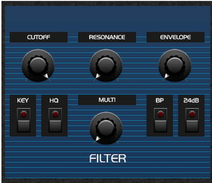
It implements a Multimode 12dB/octave filter like the Oberheim SEM module. Using the **MULTI** rotary control, you can crossfade between low-pass behavior on the complete left, to either notch (by default) or bandpass (using the BP switch) behavior at 12 o'clock, and high-pass behavior on the far right.
